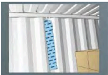
4. Hang desiccant from ceiling hooks
